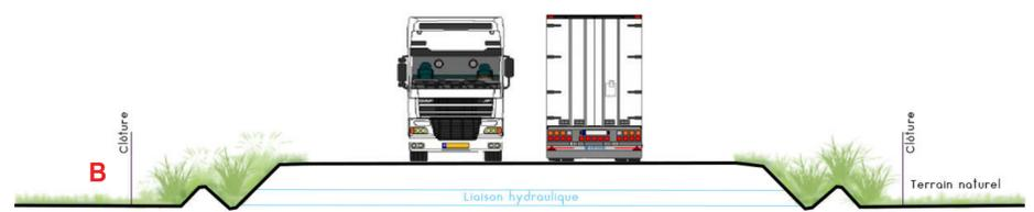
PROFIL EN TRAVERS TYPE DE LA NOUVELLE VOIE EN TRAVERSÉE DU "PRÉ NEUF". LA VOIE EST EN LÉGER REMBLAI PAR RAPPORT AUX PRAIRIES.
